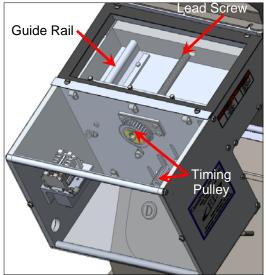
With the Valve Cover removed, you can also inspect the Thrust Bearing and the Timing Belt.
